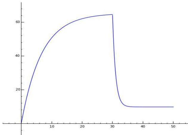
Figure 1: Velocity of falling parachutist.
