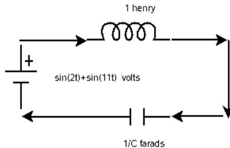
Figure 1: A simple LC circuit.
