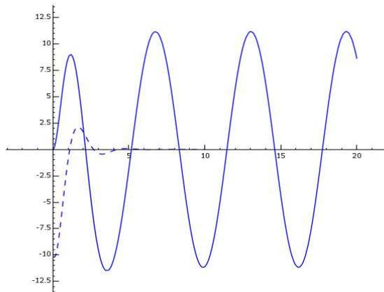
Figure 3: A LRC circuit, with damping, and the transient part (dashed) of the solution.
